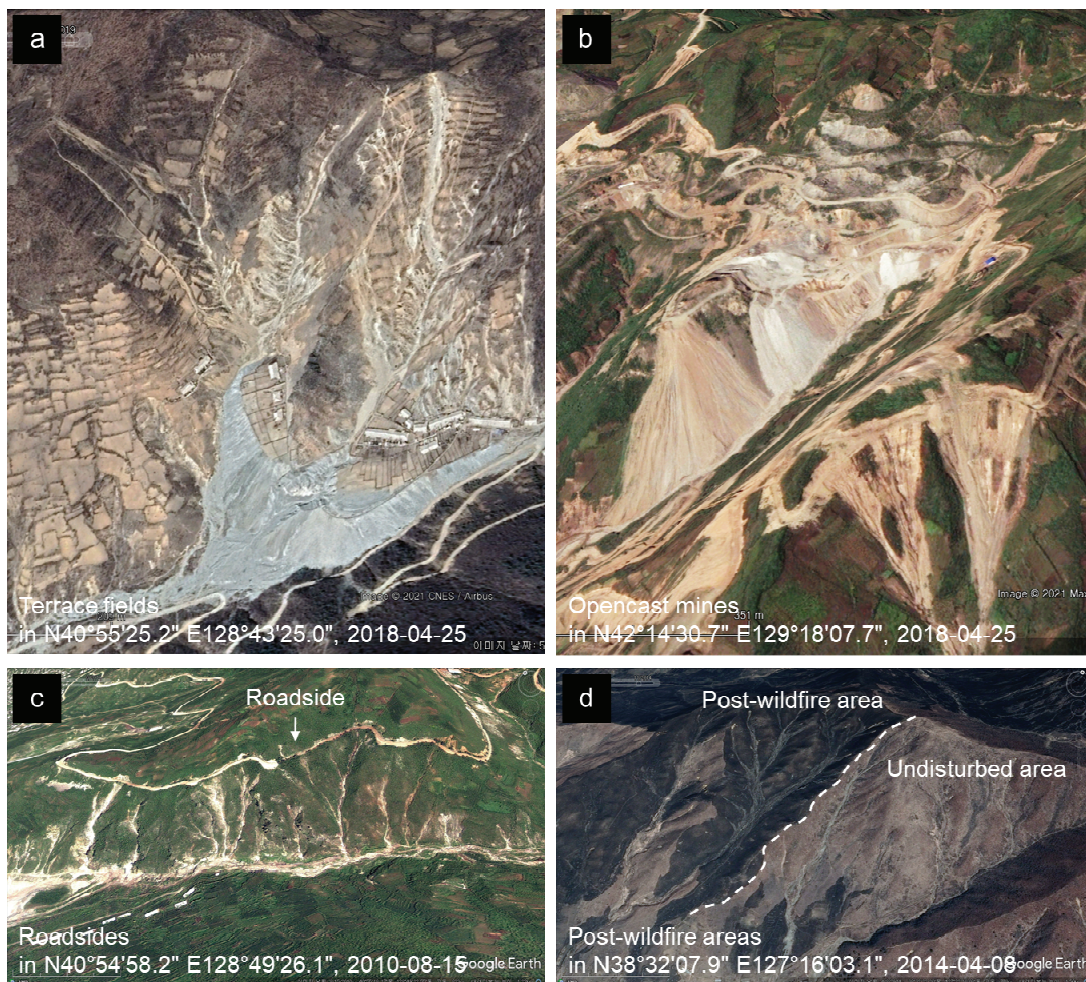
Figure 4. Examples of sediment-related disaster due to human activity in North Korea observed by Google Earth (a: terrace fields, b: opencast mines, c: roadsides, d: post-wildfire areas).
