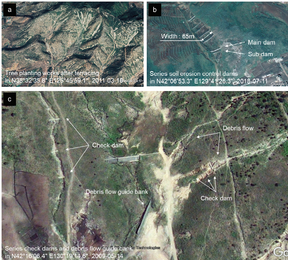
Figure 5. Examples of erosion control works in North Korea observed by Google Earth (a: tree planting works after terracing, b: a series of check dams, c: a series of check dams and debris flow guide bank).
