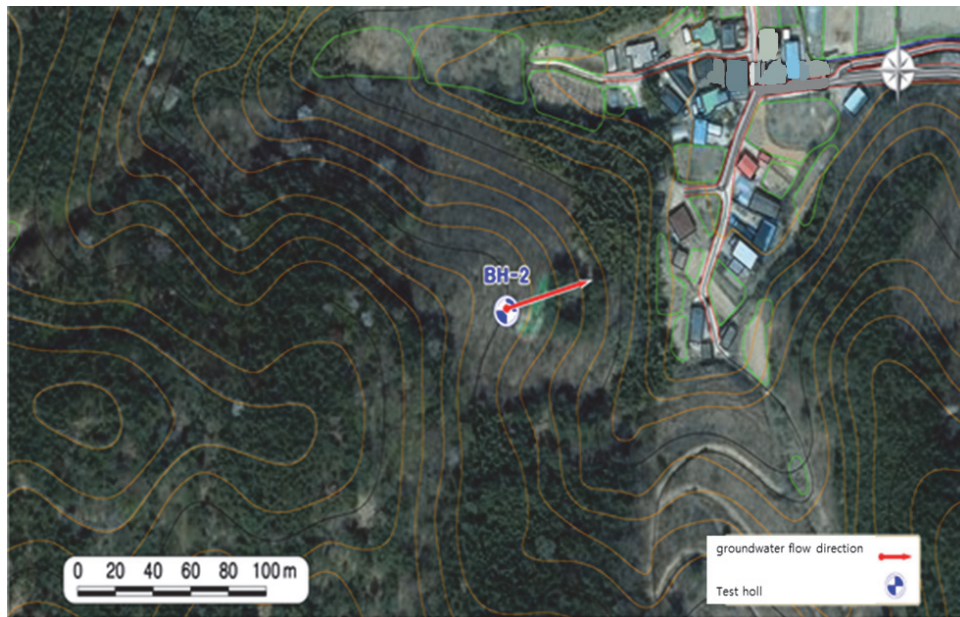
Figure 8. Groundwater flow direction through sulfur analysis according to ground investigation.
