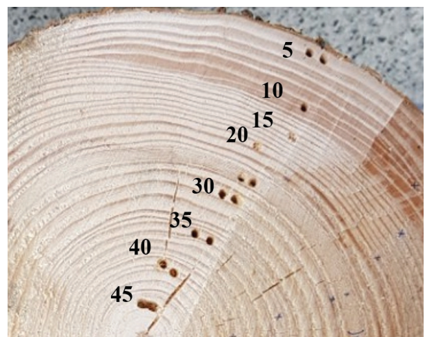
Figure 1. The crushed points along annual rings on wood disk of Pinus densiflora . The Pinus densiflora wood disk ( \varnothing = 30 cm, thickness = 8 cm), the age of which is approximately 48 years, was cut in early October 2018.
