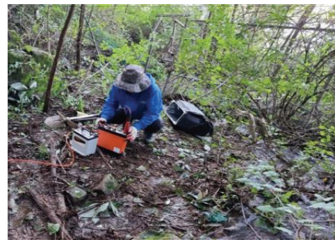
(b) Electric resistivity survey in field
