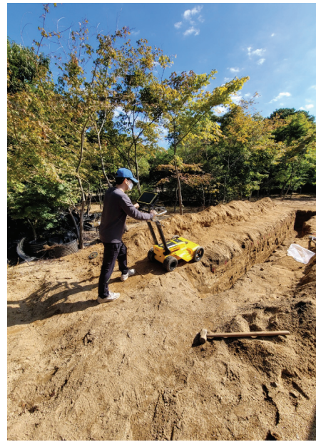
Figure 5. Photo of GPR experiment.
