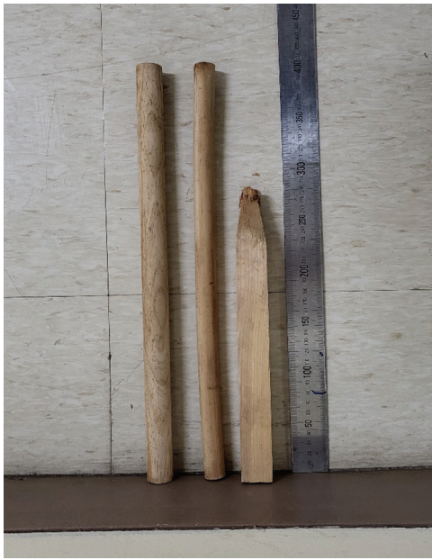
Figure 2. The model-root used in the experiment. The model-root on the left has a diameter of 2.3 cm and is cylindrical. The model-root in the middle has a diameter of 1.5 cm. The model-root on the right is a stake, having a rectangular shape with 3 by 3 cm.
