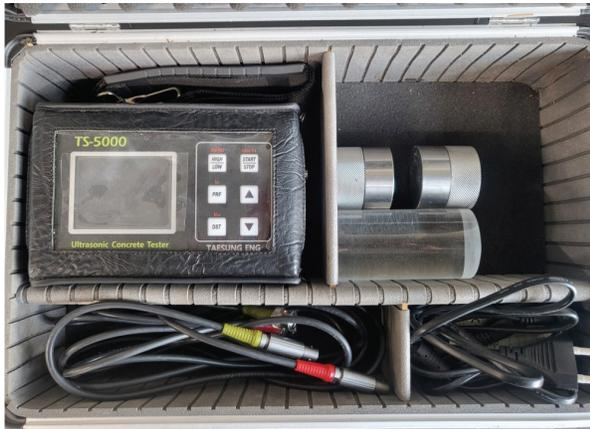
Figure 6. Ultrasonic velocity meter (TAESUNG TS-5000) for the ultrasonic pulse velocity test.
