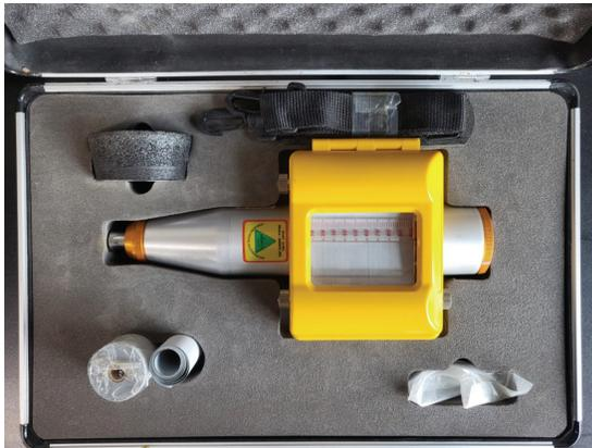
Figure 3. Concrete test hammer (SANYO NSR-2) for the rebound hardness test.
