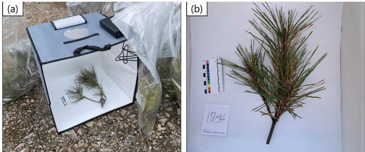
Figure 2. Setup for smartphone image acquisition: (a) a portable photobox with LED light; (b) an example image.
