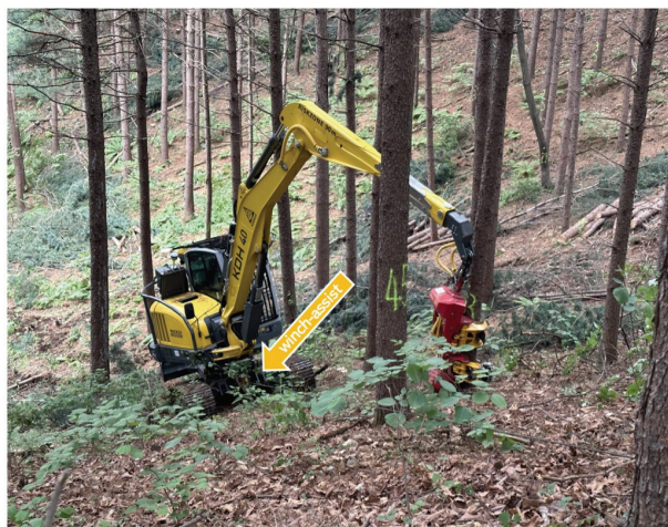
Figure 1. Harvester (KDH40-1) equipped with a winch-assist system used in this study.
