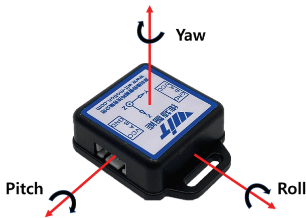
Figure 5. IMU-based Roll, Pitch, and Yaw attitude angles.
