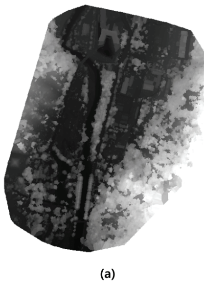
Figure 6. Digital surface model(DSM) and orthophoto generated using aerial photography; (a) Generated DSM, (b) Generated orthophoto.
